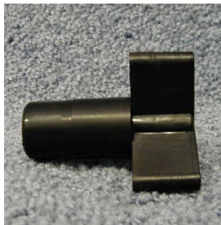
Wrench for tightening or loosening the stainless steel clamp
