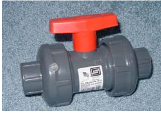
B05 007 3/4" PVC Valve With Viton 'O'Rings 235 psi
